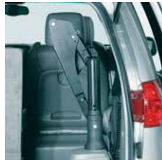
Quick release pin allows lift head to fold down.
